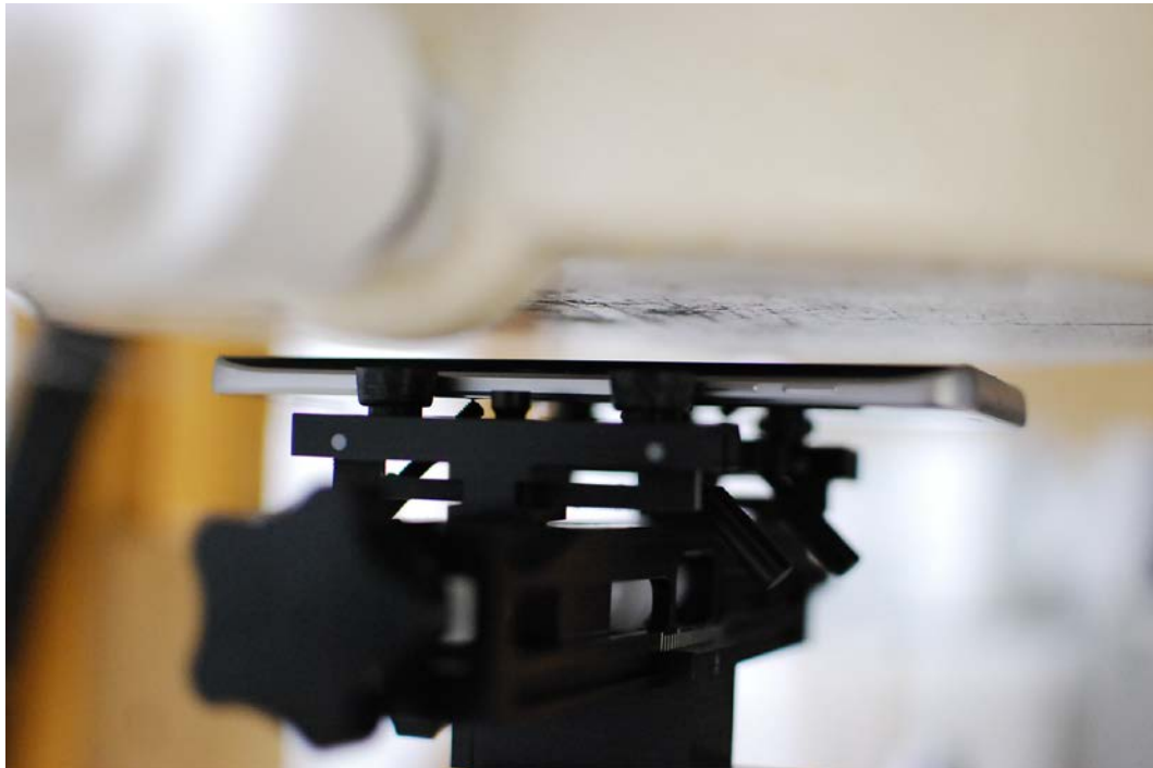
SAR Test Setup Photo 6– Back Side at 1.0 cm (Hotspot, Body-worn)
