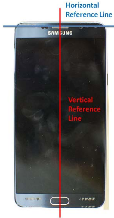
SAR Test Setup Photo 15– DUT Reference Lines
