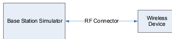
Figure 9-2 Power Measurement Setup
