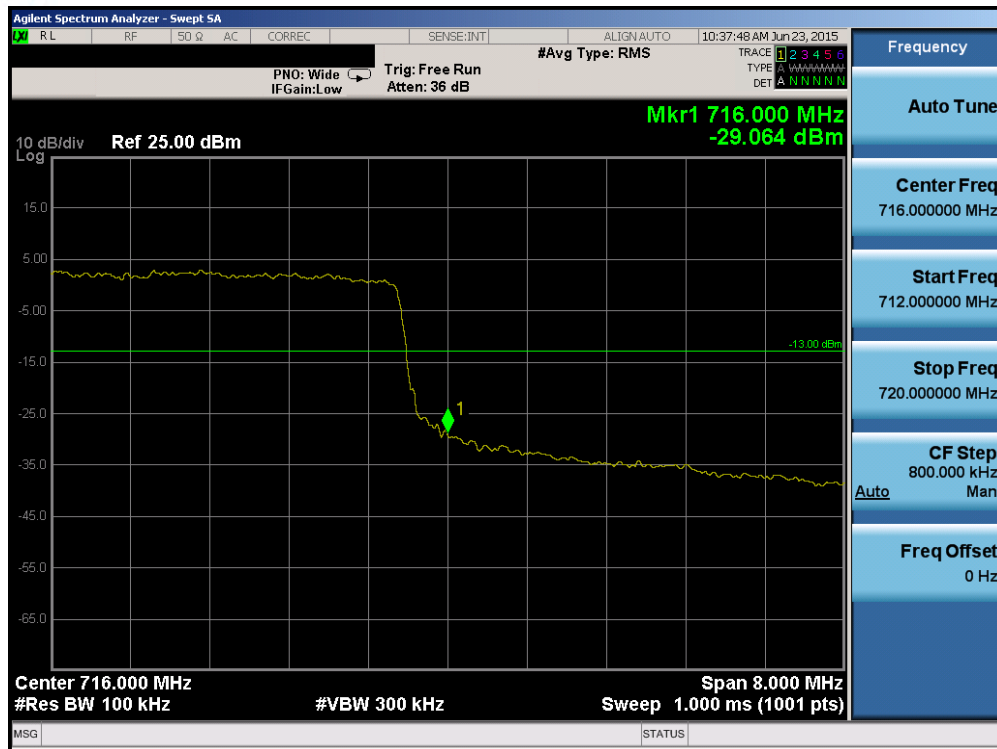
Plot 6-76. Upper Band Edge Plot (Band 17 – 10.0MHz QPSK – RB Size 50)
