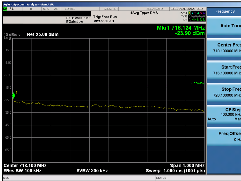
Plot 6-74. Upper Extended Band Edge Plot (Band 17 – 5.0MHz QPSK – RB Size 25)
