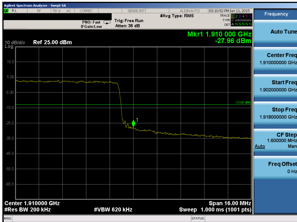
Plot 6-115. Upper Band Edge Plot (Band 2 – 20.0MHz QPSK – RB Size 100)
