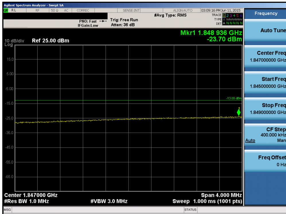
Plot 6-114. Lower Extended Band Edge Plot (Band 2 – 20.0MHz QPSK – RB Size 100)
