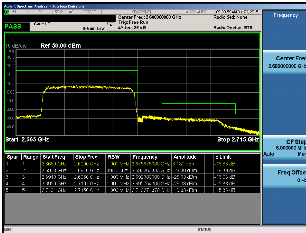
Plot 6-124. Upper ACP Plot (Band 41 – 20.0MHz QPSK – RB Size 100)
