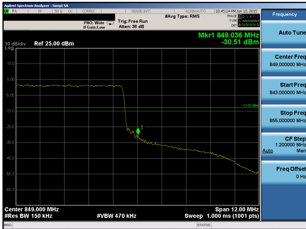
Plot 6-92. Upper Band Edge Plot (Band 26 – 15.0MHz QPSK – RB Size 75)
