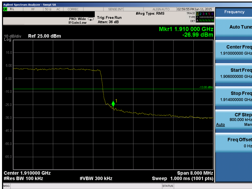
Plot 6-107. Upper Band Edge Plot (Band 2 – 10.0MHz QPSK – RB Size 50)
