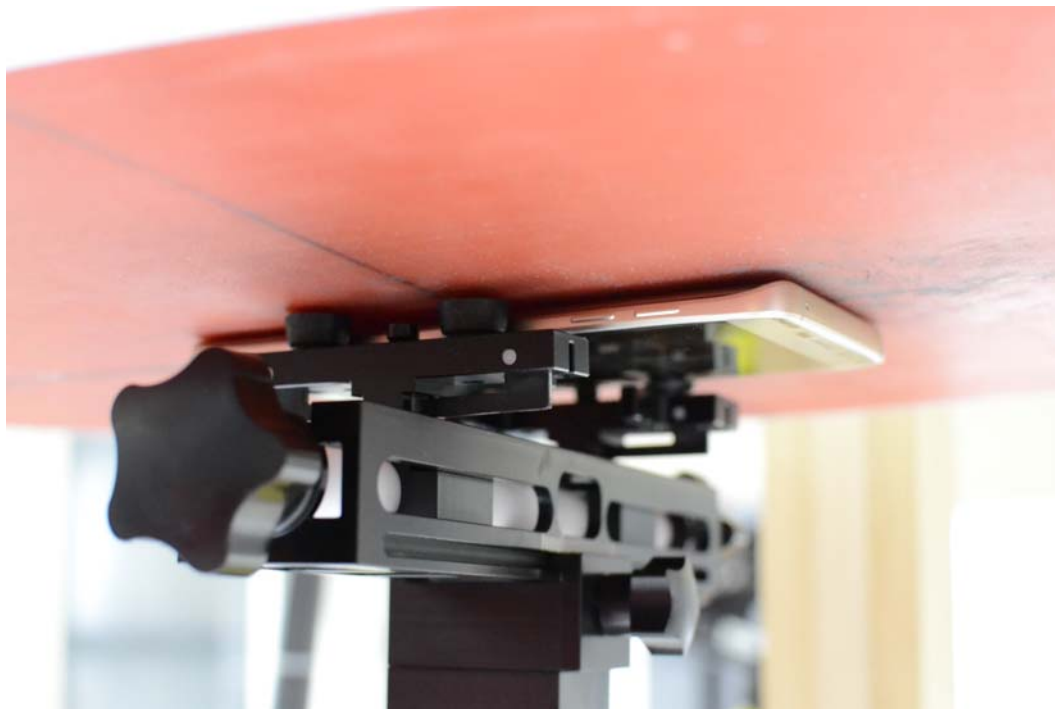
SAR Test Setup Photo 5– Back Side at 0.0 cm (Extremity)
