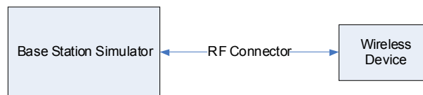
Figure 10 Power Measurement Setup
