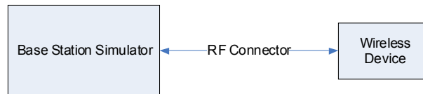
Figure 12 Power Measurement Setup
