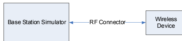
Figure 10 Power Measurement Setup
