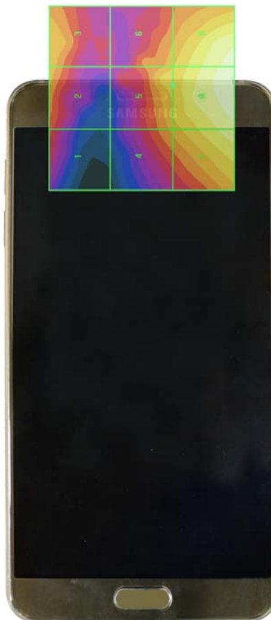
Figure 18-4 E-Field WD Scan overlay
