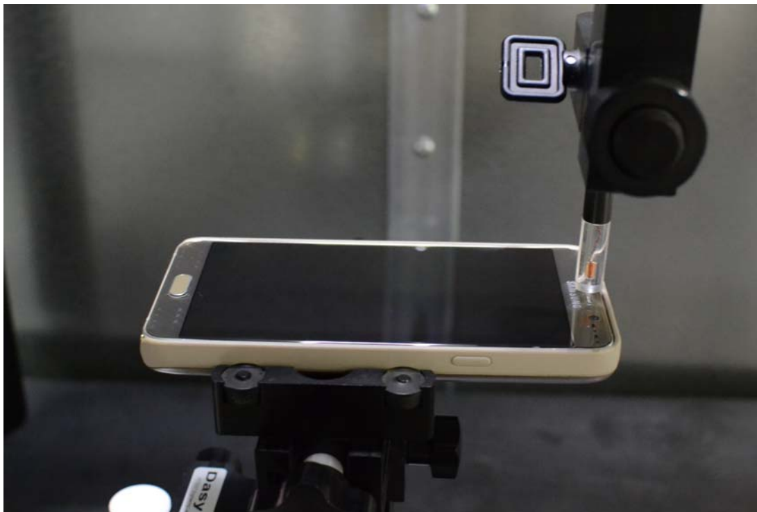
Figure 12-1 Test Setup for Wireless Device
