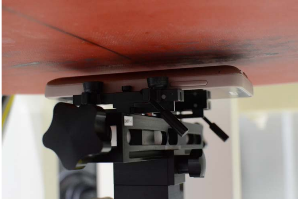
SAR Test Setup Photo 5 – Back Side at 1.0 cm (Hotspot)
