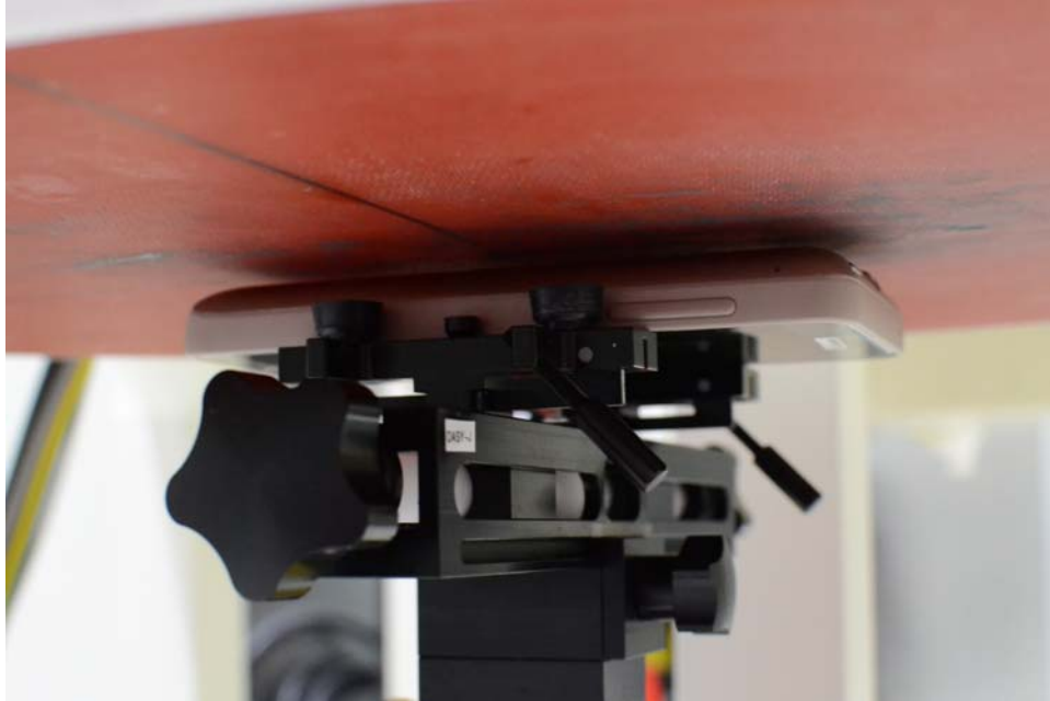
SAR Test Setup Photo 3 – Back Side at 0.3 cm (Phablet)
