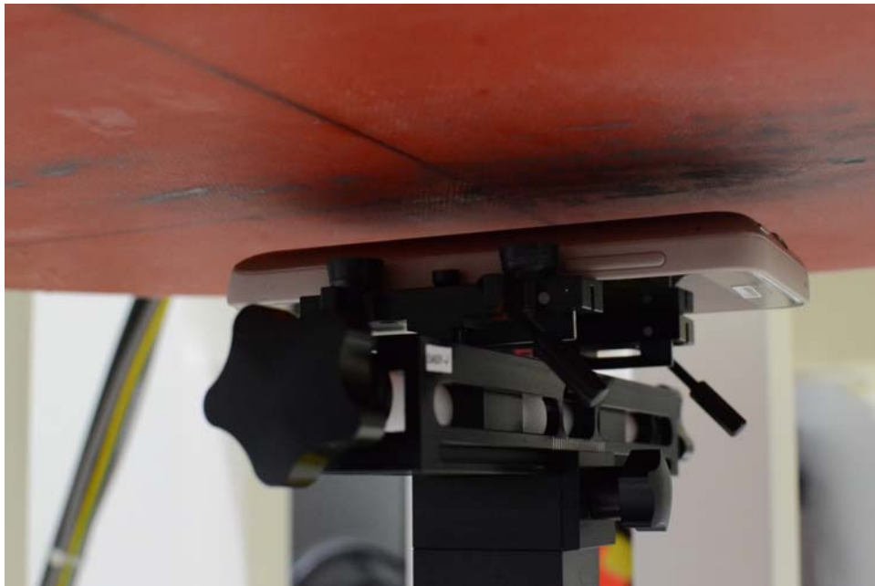
SAR Test Setup Photo 4 – Back Side at 1.5 cm (Body-worn)
