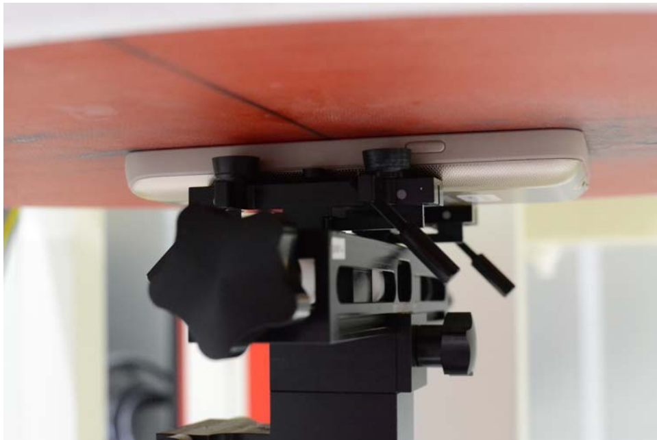
SAR Test Setup Photo 6 — Front Side at 0.0 cm (Phablet)
