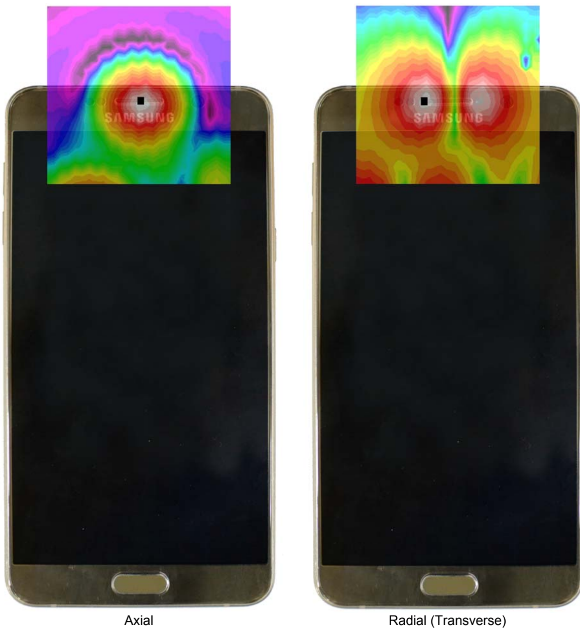
Figure 13-3 T-Coil Scan Overlay Magnetic Field Distributions
