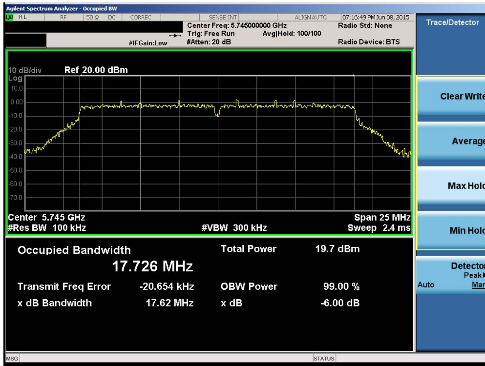
Plot 6-71. 6dB Bandwidth Plot (20MHz BW 802.11n (UNII Band 3) – Ch. 149)
