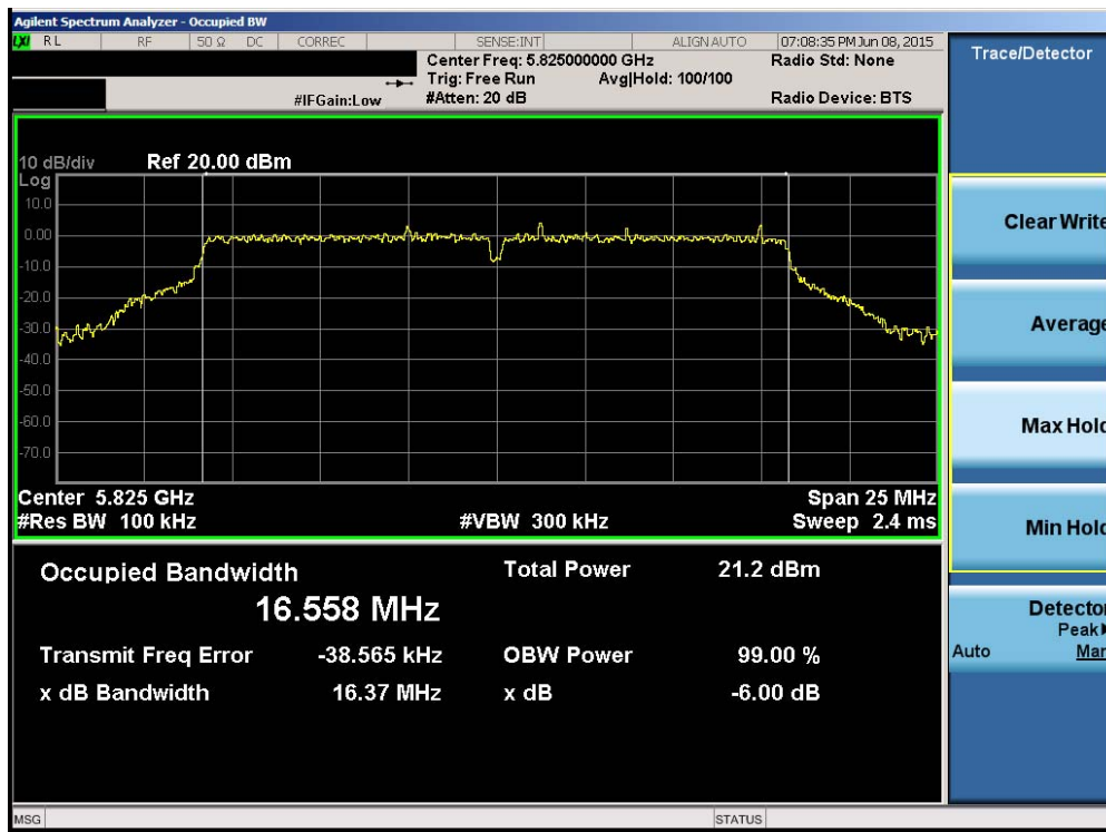
Plot 6-70. 6dB Bandwidth Plot (802.11a (UNII Band 3) – Ch. 165)
