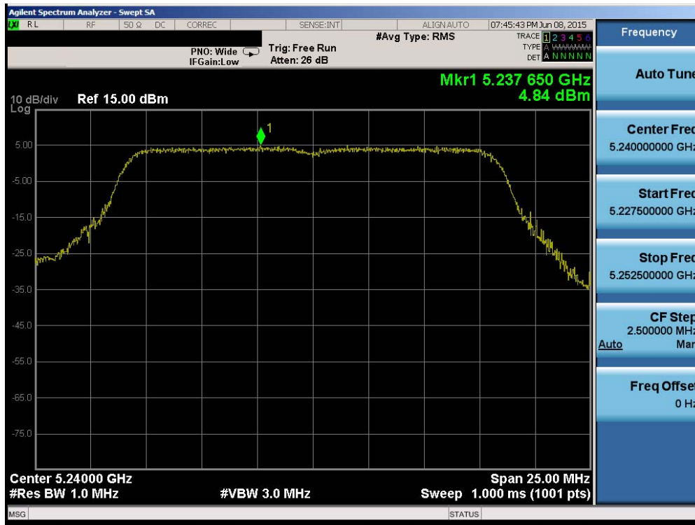
Plot 6-79. Power Spectral Density Plot (802.11a (UNII Band 1) – Ch. 48)
