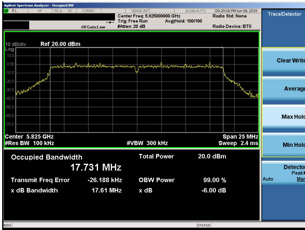
Plot 6-64. 6dB Bandwidth Plot (20MHz BW 802.11n (UNII Band 3) – Ch. 165)
