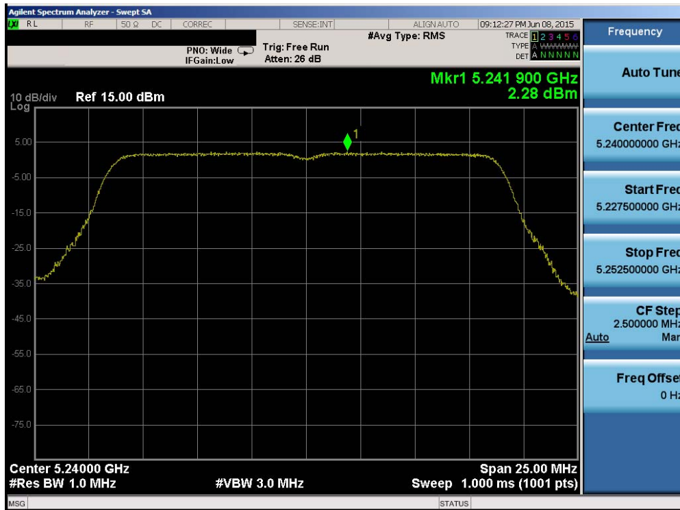
Plot 6-82. Power Spectral Density Plot (20MHz BW 802.11n (UNII Band 1) – Ch. 48)
