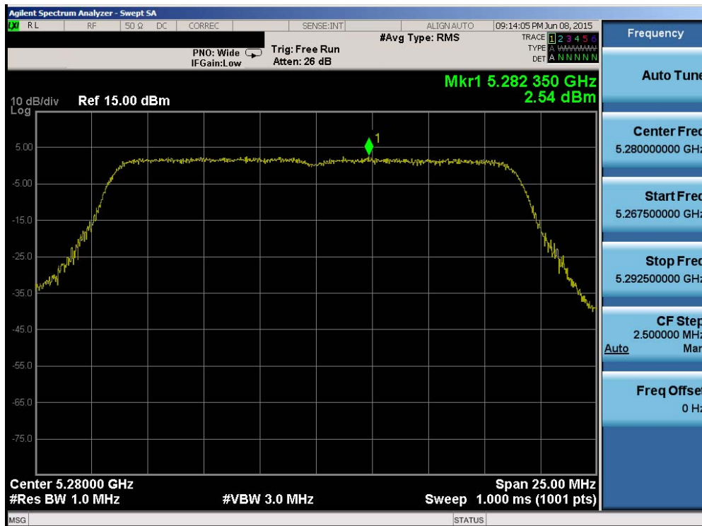
Plot 6-90. Power Spectral Density Plot (20MHz BW 802.11n (UNII Band 2A) – Ch. 56)
