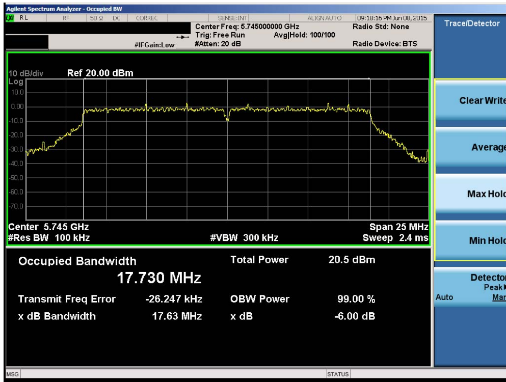
Plot 6-62. 6dB Bandwidth Plot (20MHz BW 802.11n (UNII Band 3) – Ch. 149)
