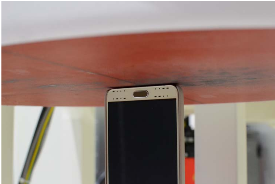
SAR Test Setup Photo 6 – Bottom Edge at 0.0 cm (Phablet)
