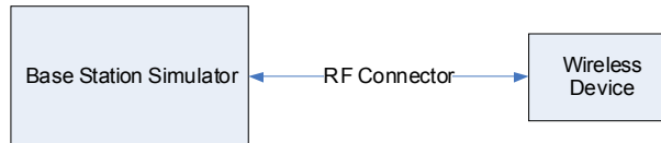
Figure 9-1 Power Measurement Setup
