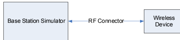
Figure 9-3 Power Measurement Setup
