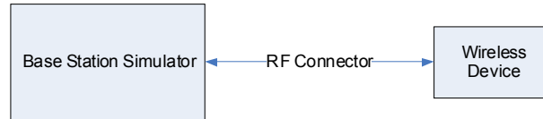
Figure 9-2 Power Measurement Setup
