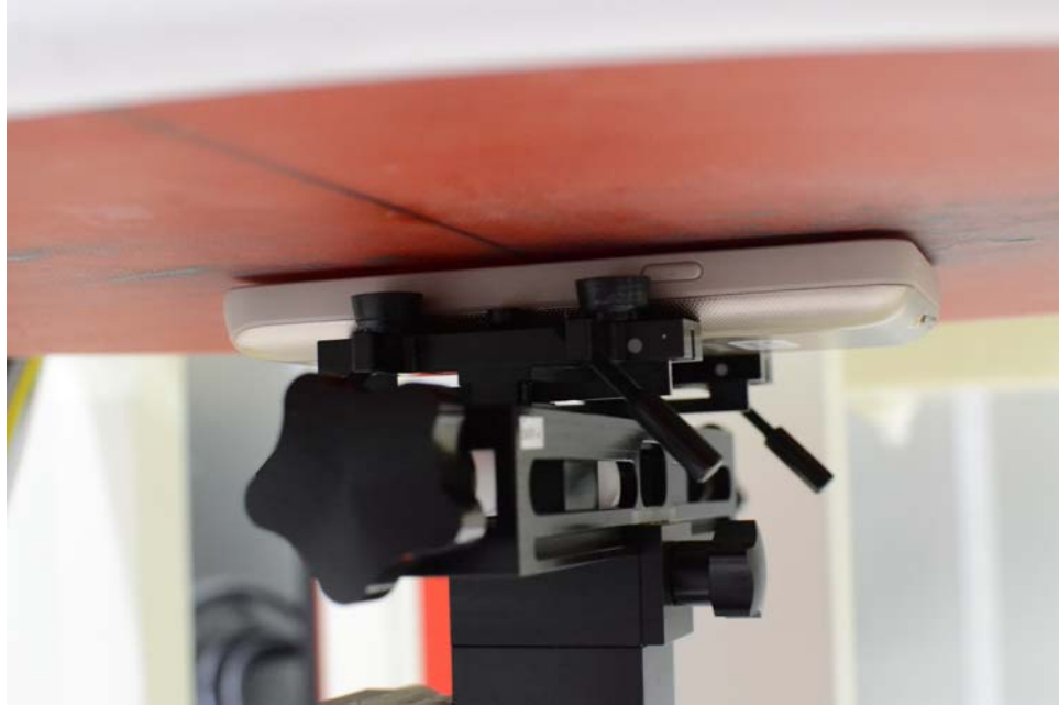
SAR Test Setup Photo 7 — Front Side at 0.1 cm (Phablet)
