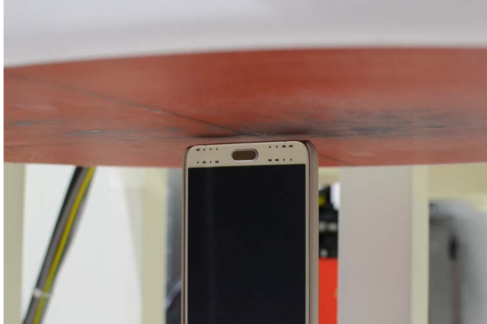
SAR Test Setup Photo 9 – Bottom Edge at 0.4 cm (Phablet)
