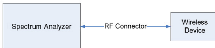
Figure 6-1. Test Instrument & Measurement Setup
