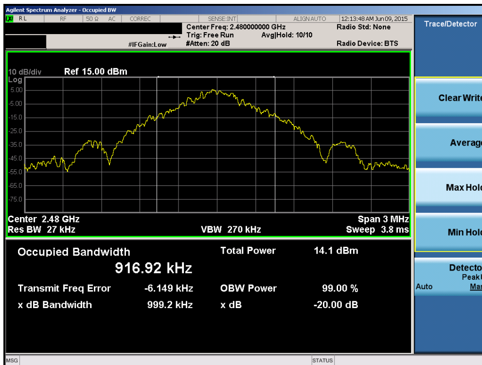
Plot 6-3. 20dB Bandwidth Plot (Bluetooth, 1Mbps – Ch. 78)
