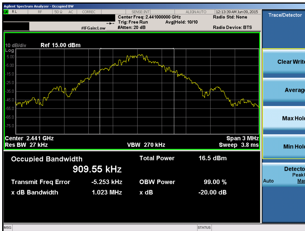
Plot 6-2. 20dB Bandwidth Plot (Bluetooth, 1Mbps – Ch. 39)
