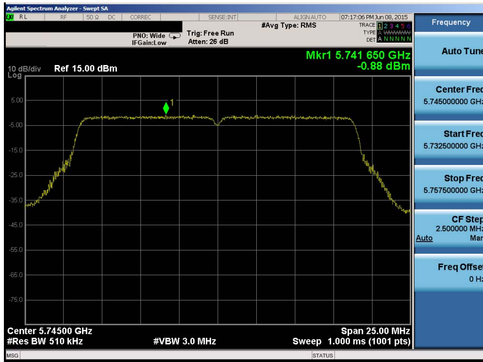
Plot 6-147. Power Spectral Density Plot (20MHz BW 802.11n (UNII Band 3) – Ch. 149)
