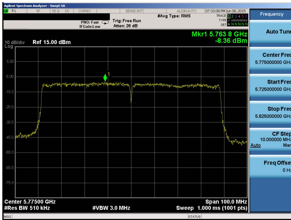
Plot 6-152. Power Spectral Density Plot (80MHz BW 802.11ac (UNII Band 3) – Ch. 155)
