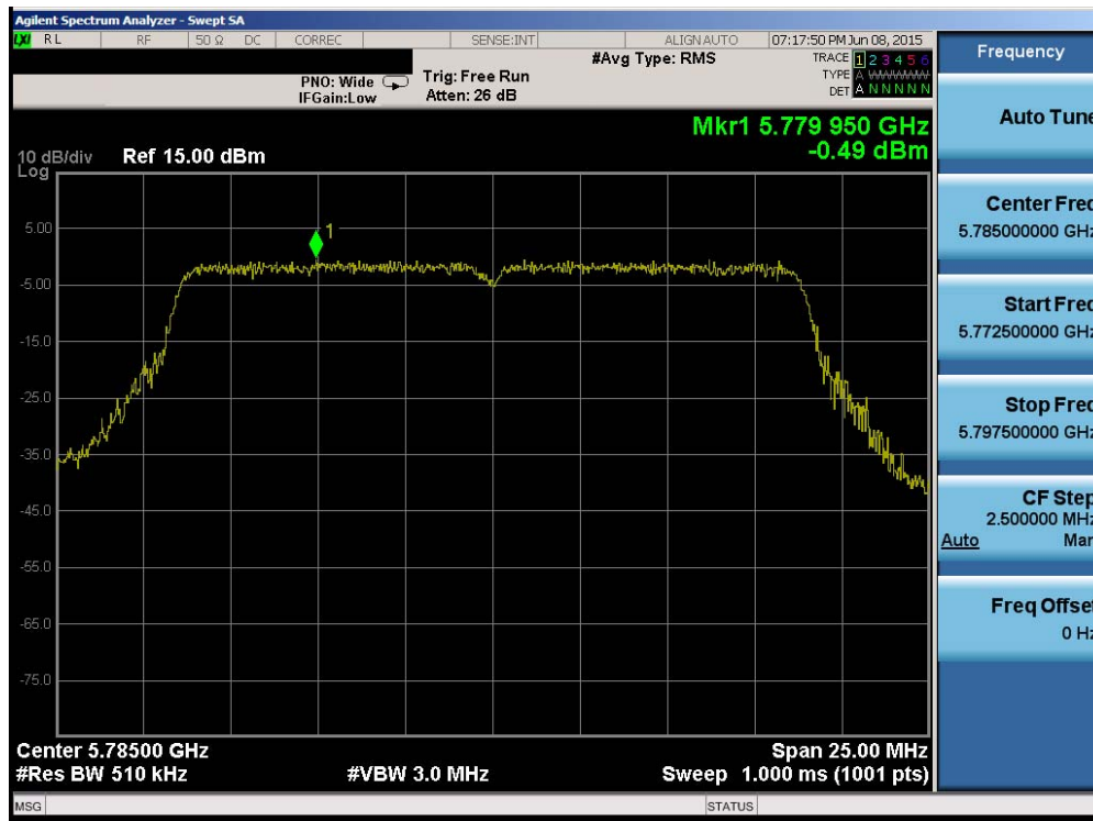
Plot 6-148. Power Spectral Density Plot (20MHz BW 802.11n (UNII Band 3) – Ch. 157)
