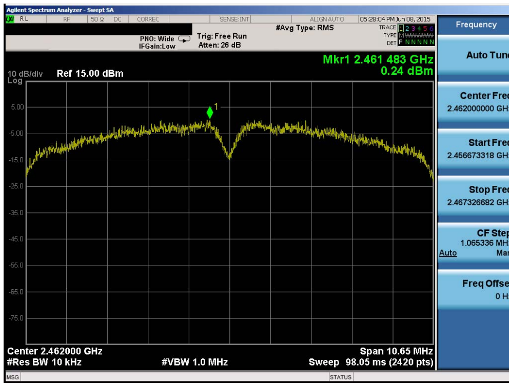
Plot 6-21. Power Spectral Density Plot (802.11b – Ch. 11)
