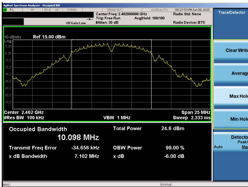
Plot 6-3. 6dB Bandwidth Plot (802.11b – Ch. 11)
