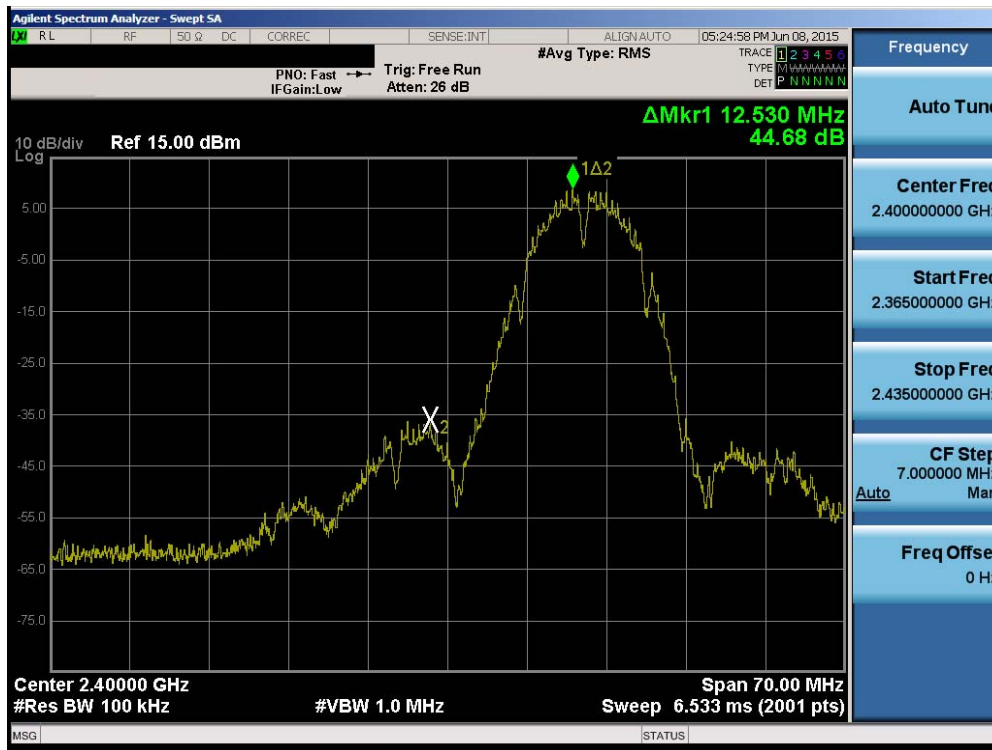
Plot 6-37. Band Edge Plot (802.11b – Ch. 1)
