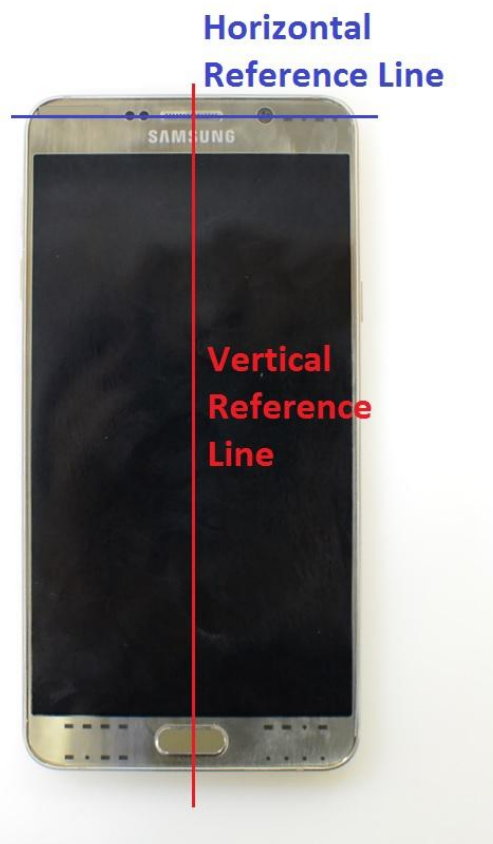
SAR Test Setup Photo 21– DUT Reference Lines
