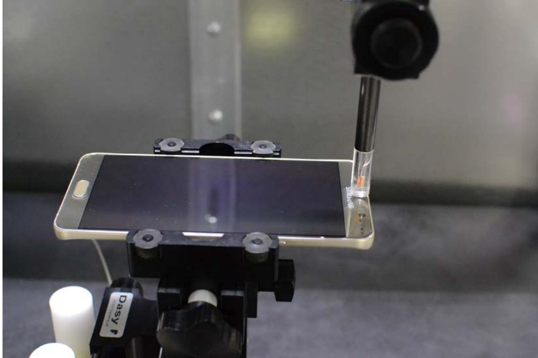
Figure 14-1 Test Setup for Wireless Device
