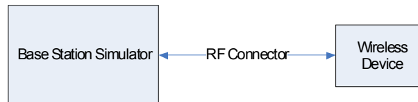
Figure 9-1 Power Measurement Setup
