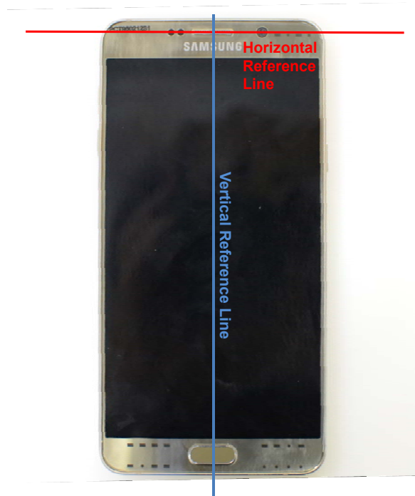
SAR Test Setup Photo 21– DUT Reference Lines
