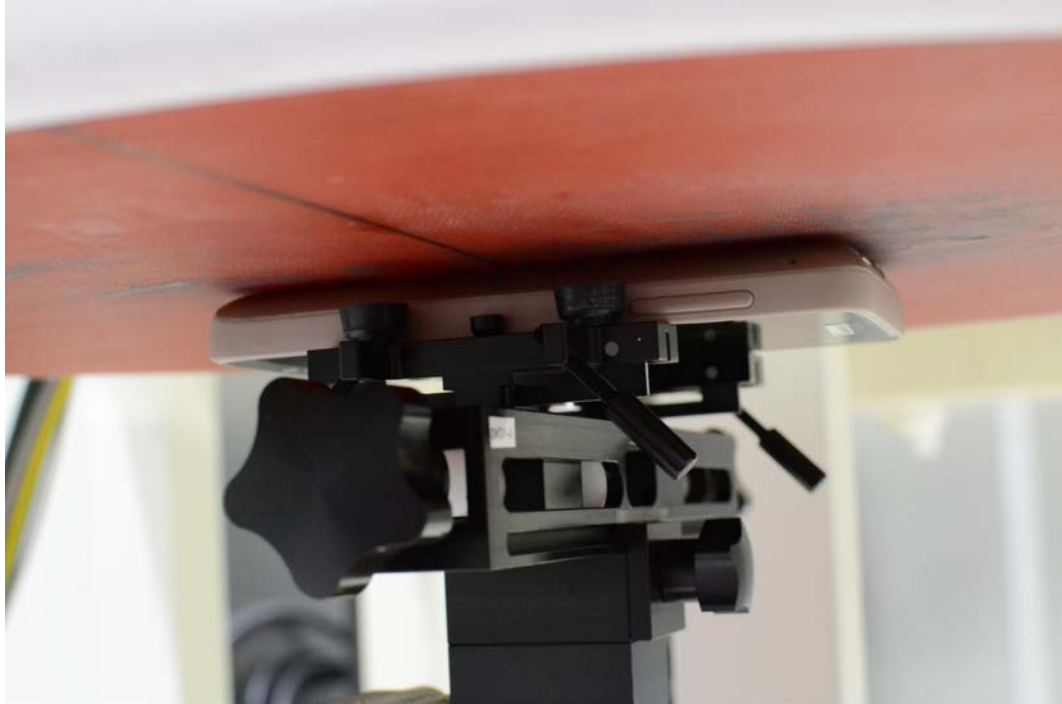
SAR Test Setup Photo 3– Back Side at 0.0 cm (Phablet)
