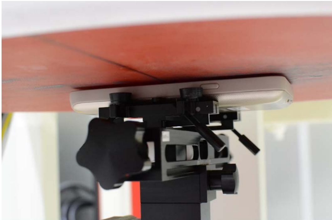
SAR Test Setup Photo 8— Front Side at 0.1 cm (Phablet)
