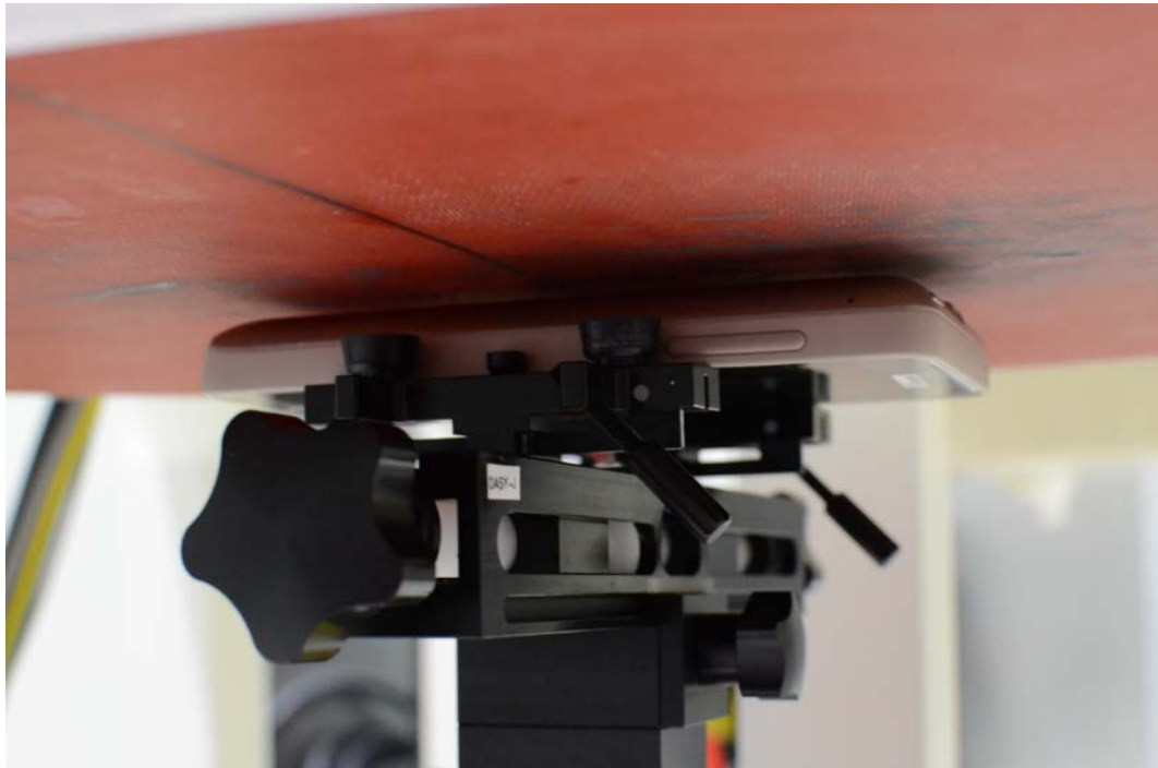
SAR Test Setup Photo 4– Back Side at 0.3 cm (Phablet)
