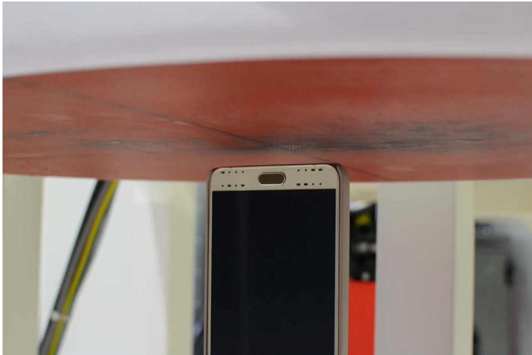
SAR Test Setup Photo 10– Bottom Edge at 1.0 cm (Hotspot)
