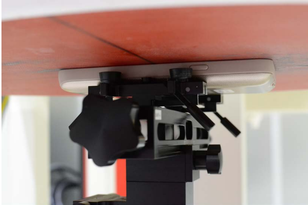
SAR Test Setup Photo 9— Front Side at 0.0 cm (Phablet)
