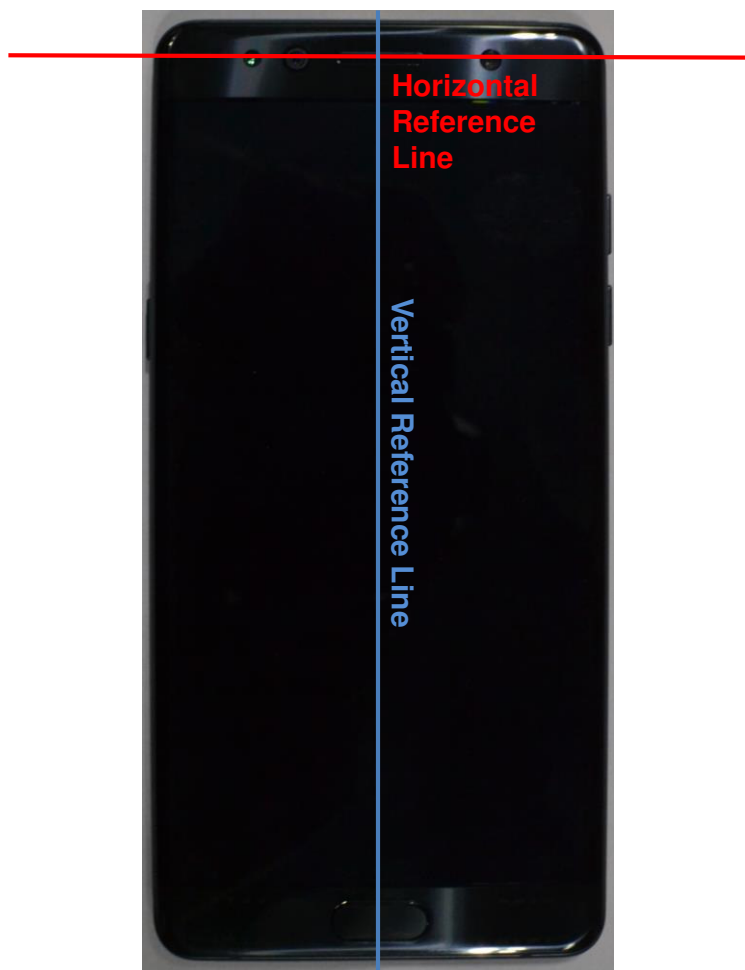
SAR Test Setup Photo 16: Horizontal and Vertical Reference Lines
