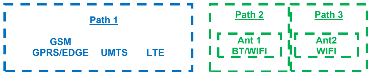
Figure 1-1 Simultaneous Transmission Paths
