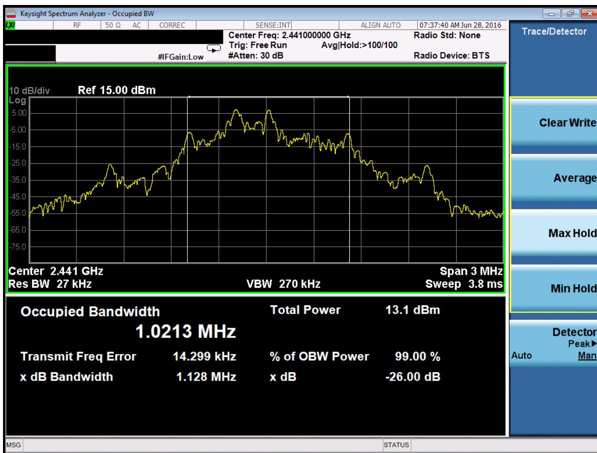
Plot 7-1. Occupied Bandwidth Plot (ANT+ – Ch. 39)
