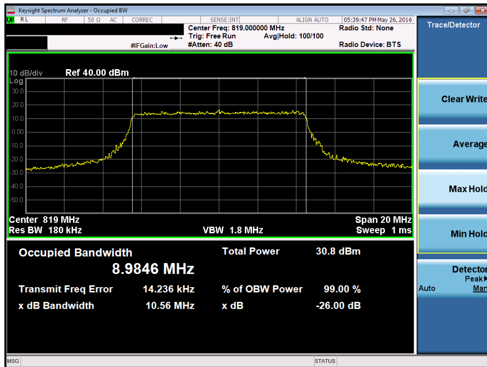
Plot 7-8. Occupied Bandwidth Plot (10MHz 16-QAM – RB Size 50)
