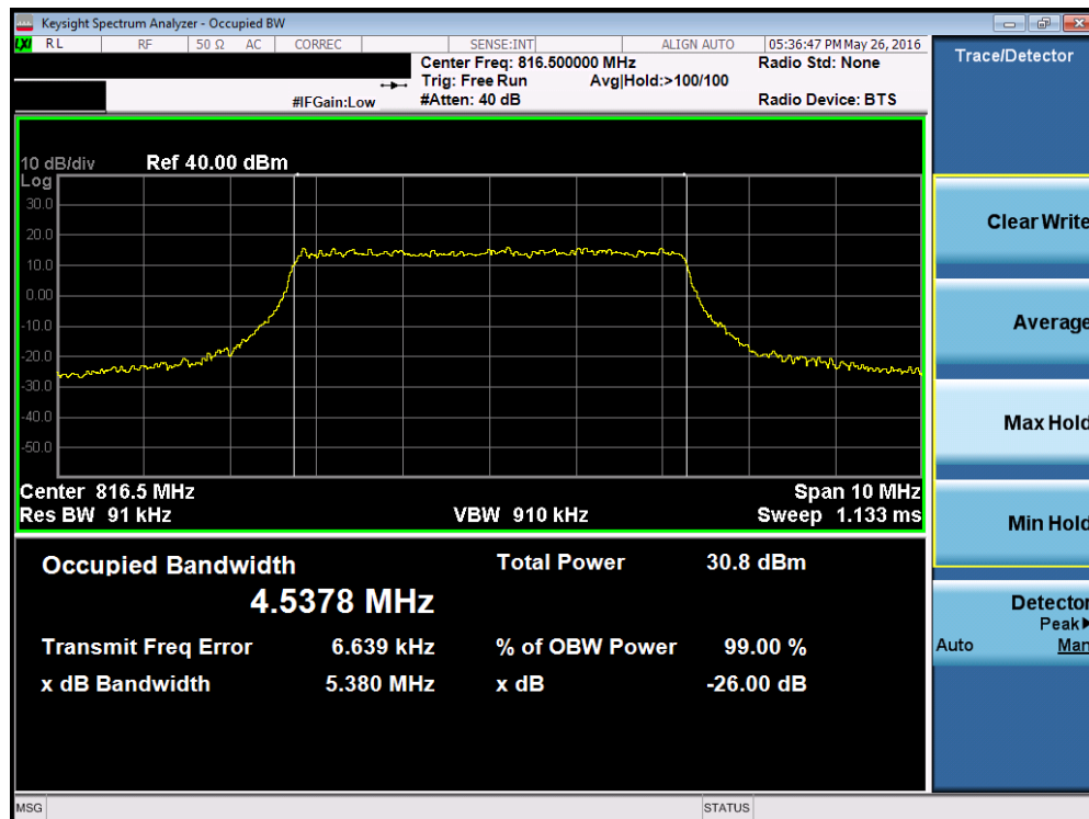
Plot 7-6. Occupied Bandwidth Plot (5MHz 16-QAM – RB Size 25– Low Channel)
