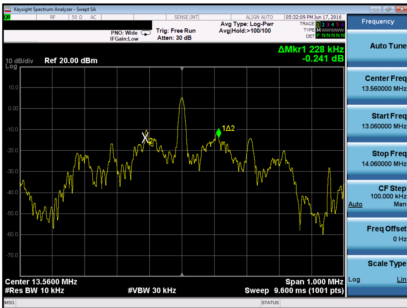
Figure 8-2. 20dB Bandwidth Plot
