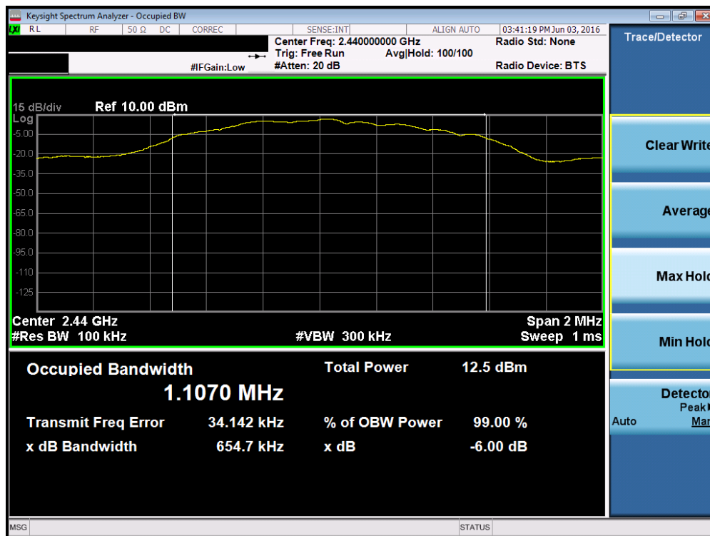
Plot 7-2. 6dB Bandwidth Plot (Bluetooth (LE) – Ch. 19)
