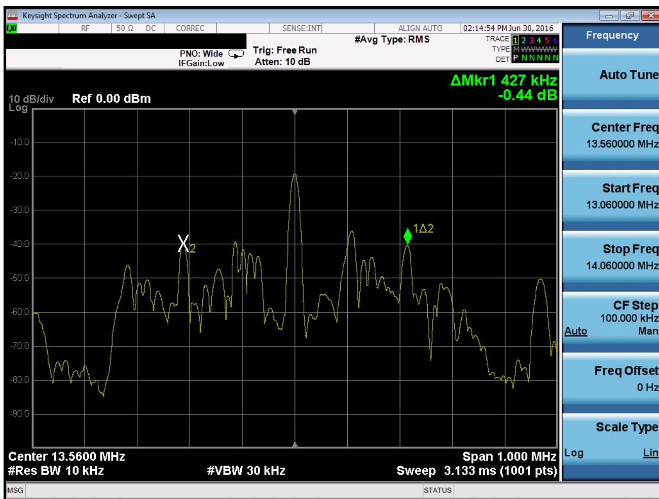
Figure 8-2. 20dB Bandwidth Plot
