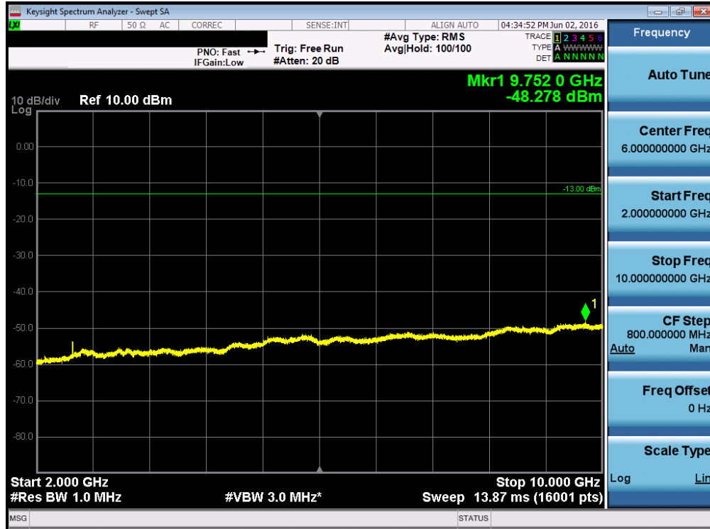
Plot 7-19. Conducted Spurious Plot (Cellular WCDMA Mode – Ch. 4183)
