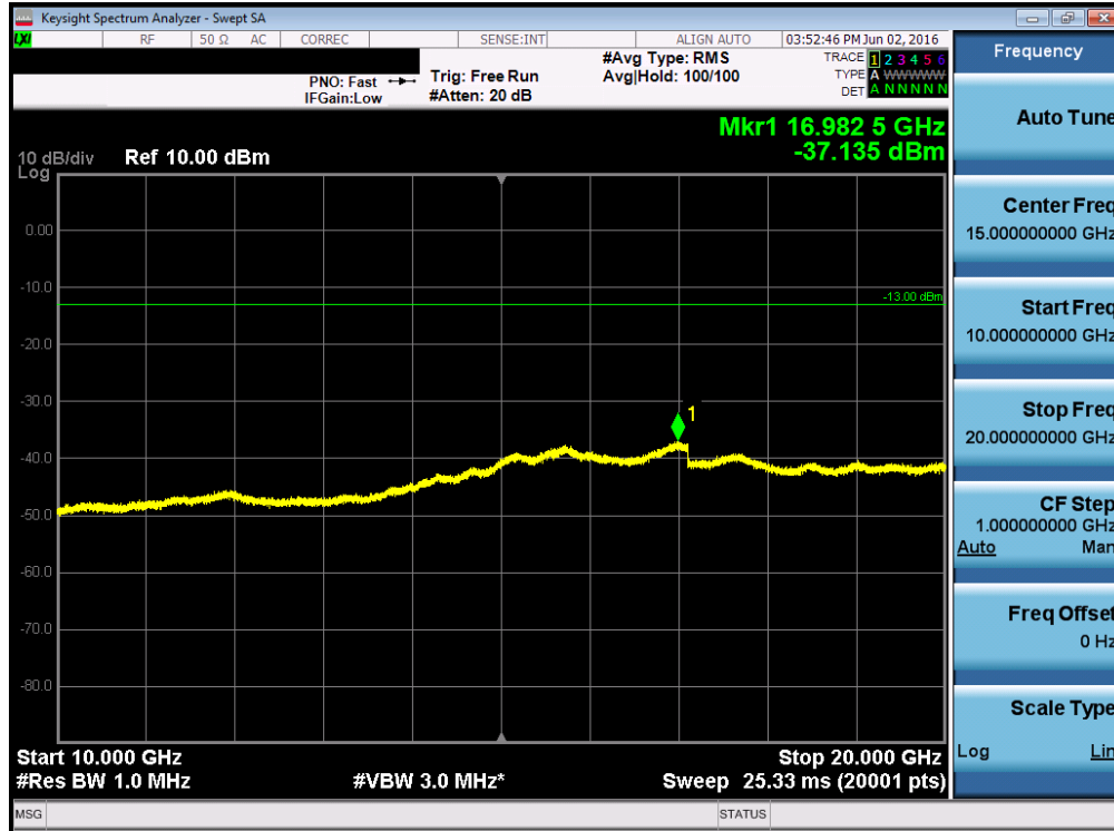
Plot 7-25. Conducted Spurious Plot (PCS WCDMA Mode – Ch. 9262)
