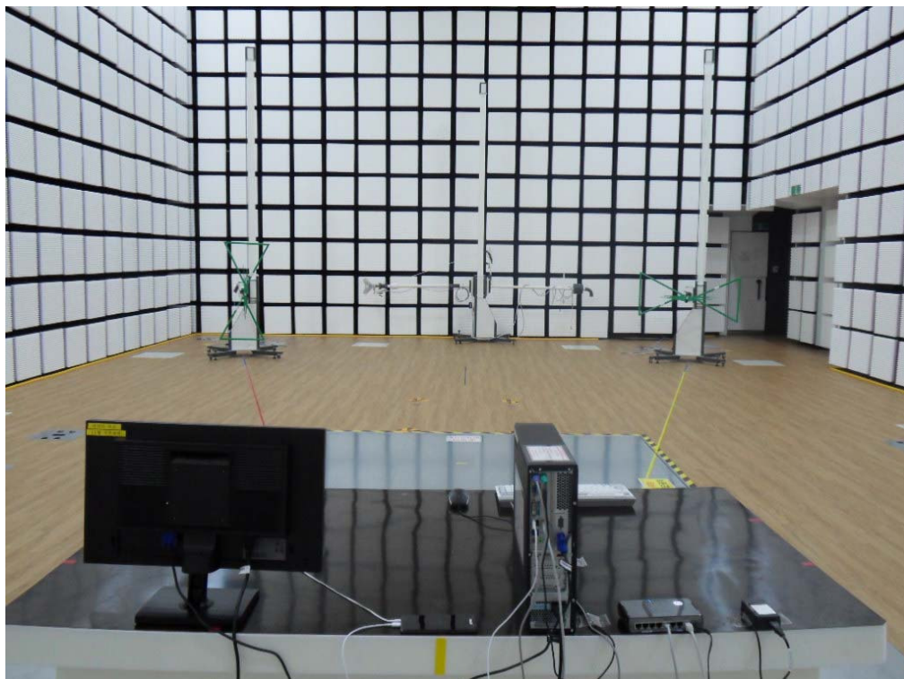
[ Radiated Disturbance for Below 1 GHz – Rear ]
