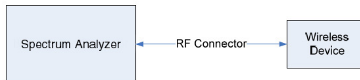
Figure 7-1. Test Instrument & Measurement Setup
