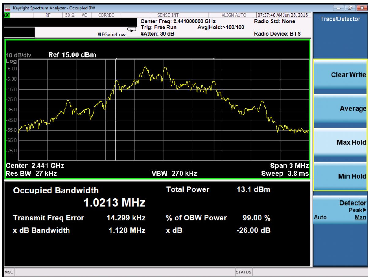
Plot 7-1. Occupied Bandwidth Plot (ANT+ – Ch. 39)
