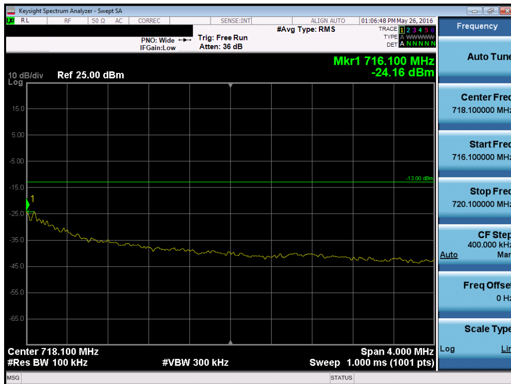
Plot 7-163. Upper Extended Band Edge Plot (Band 12/17 – 5.0MHz QPSK – RB Size 25)
