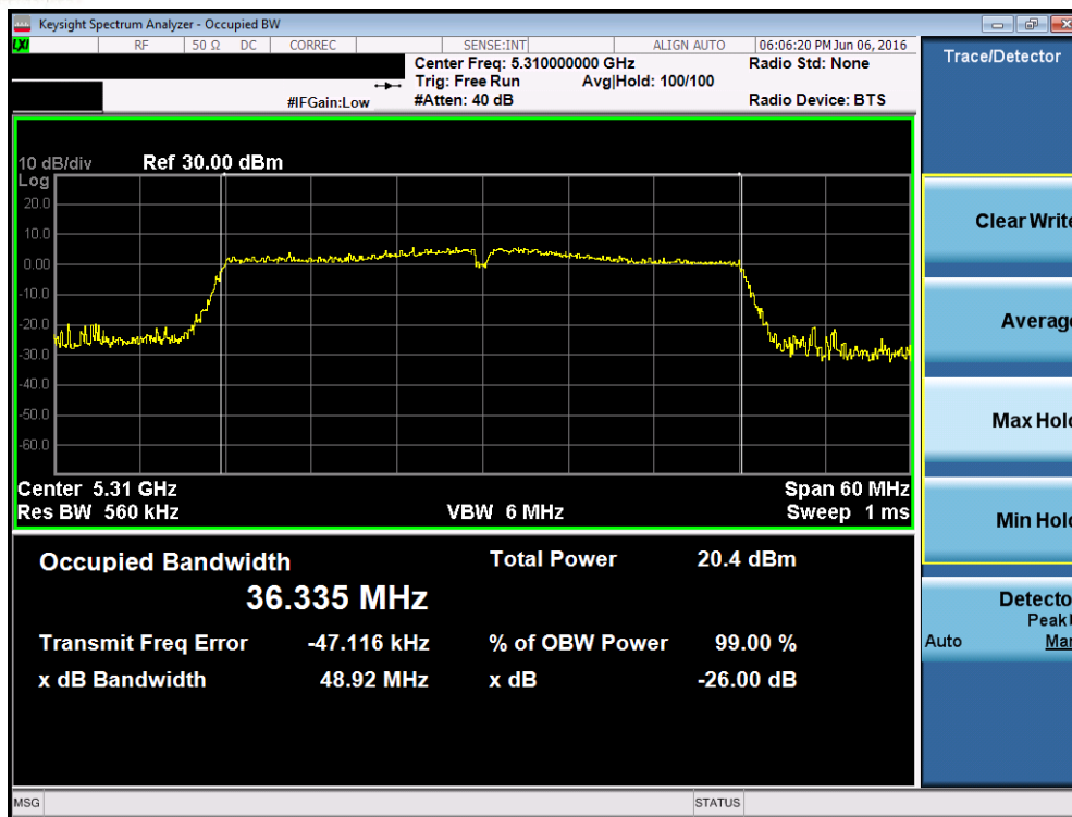
Plot 7-47. 26dB Bandwidth Plot (40MHz BW 802.11n (UNII Band 2A) – Ch. 62)
