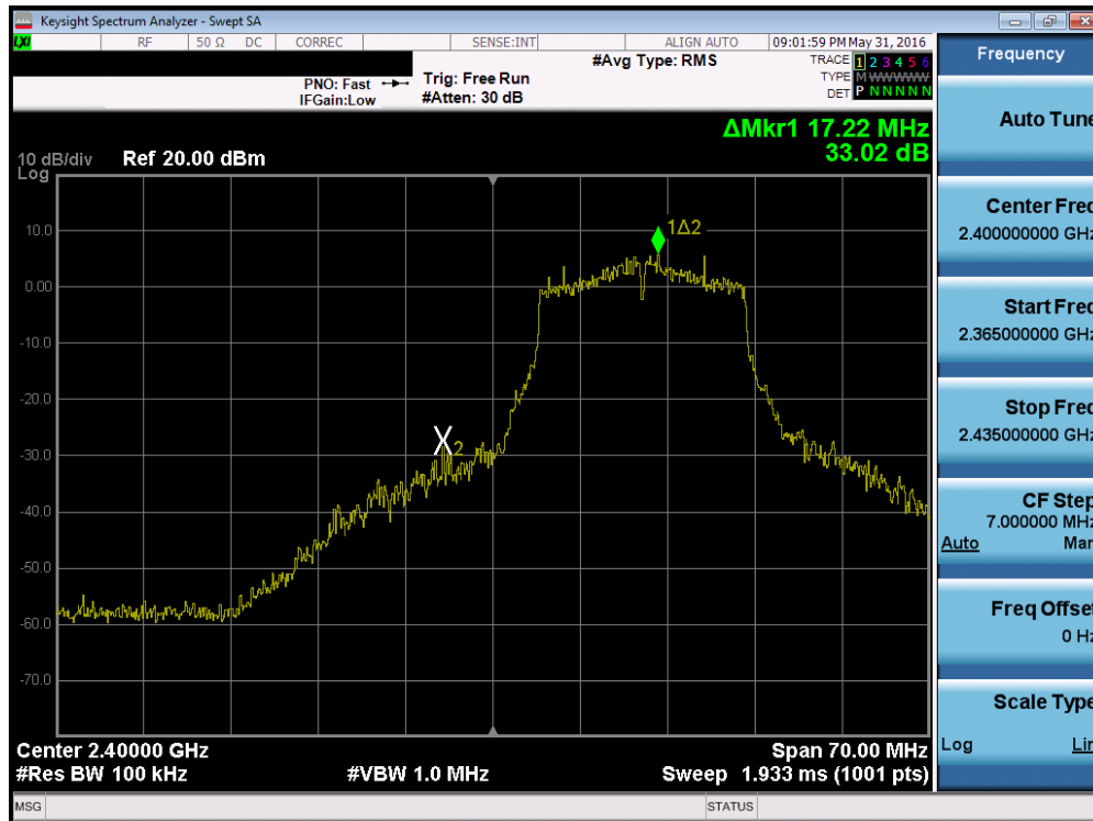
Plot 7-53. Band Edge Plot (802.11g– Ch. 1)
