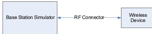
Figure 9-2 Power Measurement Setup
