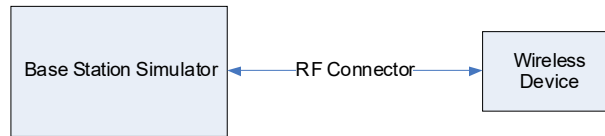
Figure 9-2 Power Measurement Setup
