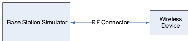
Figure 9-1 Power Measurement Setup
