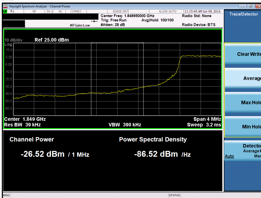
Plot 7-147. Lower Extended Band Edge Plot (Band 25 – 1.4MHz QPSK – RB Size 6)
