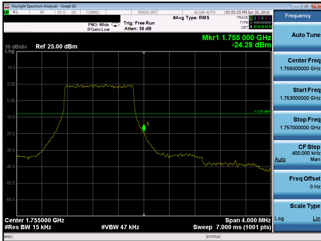
Plot 7-124. Upper Band Edge Plot (Band 4 – 1.4MHz QPSK – RB Size 6)
