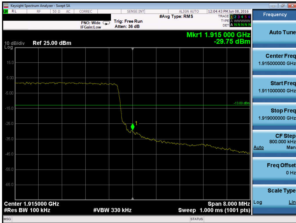
Plot 7-160. Upper Band Edge Plot (Band 25 – 10.0MHz QPSK – RB Size 50)
