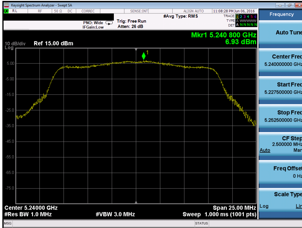
Plot 7-116. Power Spectral Density Plot (802.11a (UNII Band 1) – Ch. 48)
