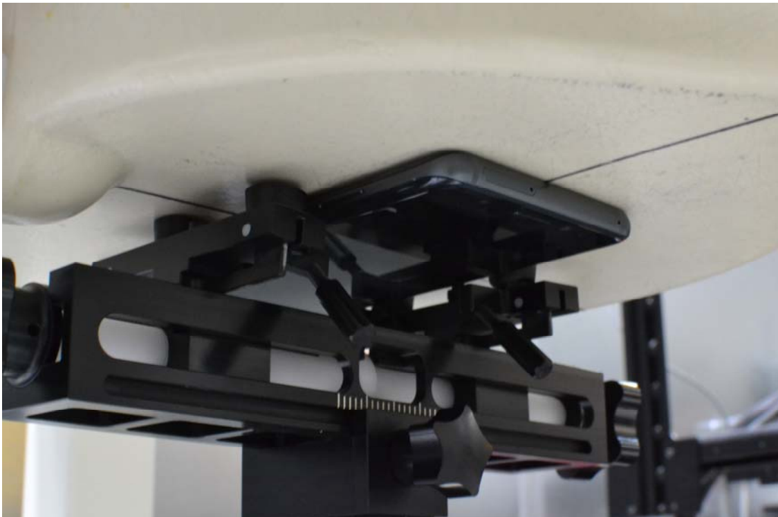
SAR Test Setup Photo 6: Back Side @ 0 mm
