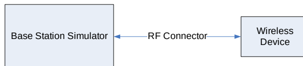
Figure 9-2 Power Measurement Setup
