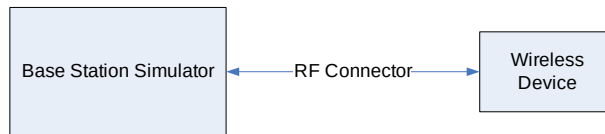
Figure 9-4 Power Measurement Setup
