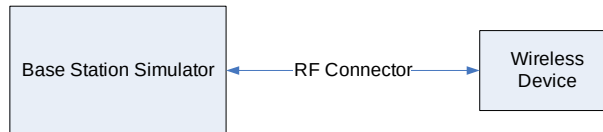
Figure 9-5 Power Measurement Setup
