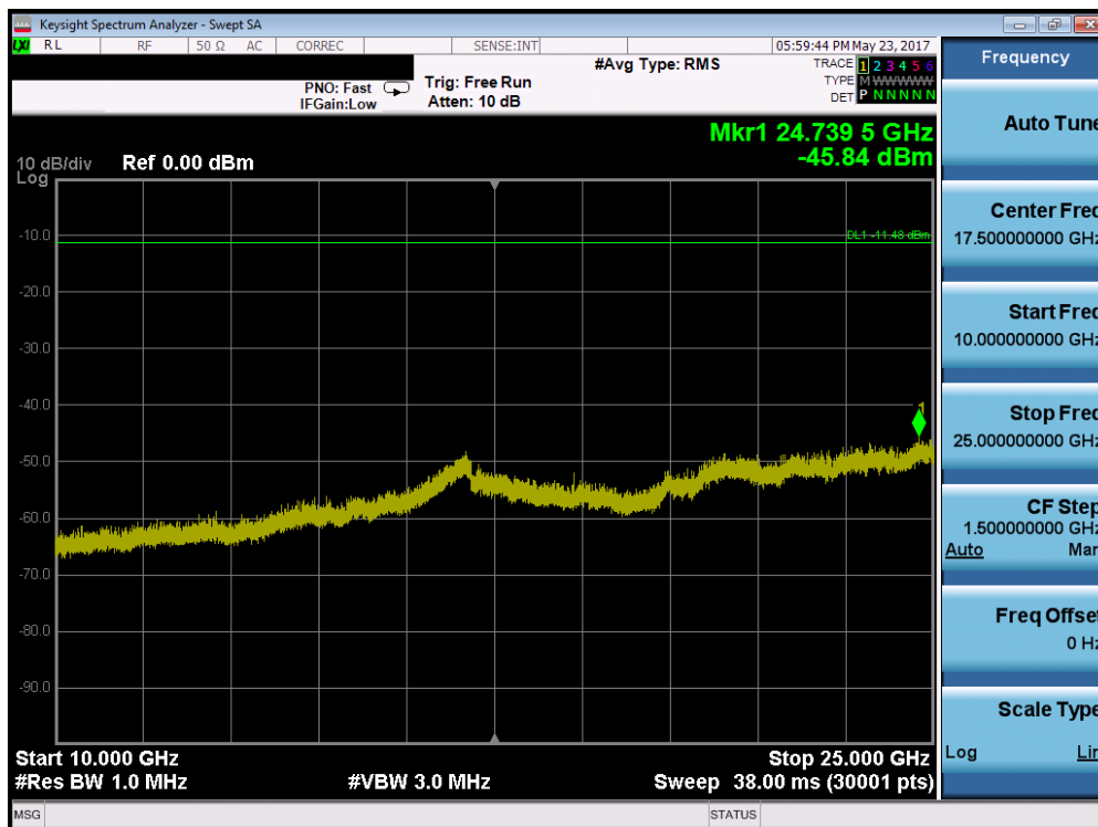
Plot 7-30. Conducted Spurious Plot (Bluetooth (LE), 2Mbps – Ch. 19)
