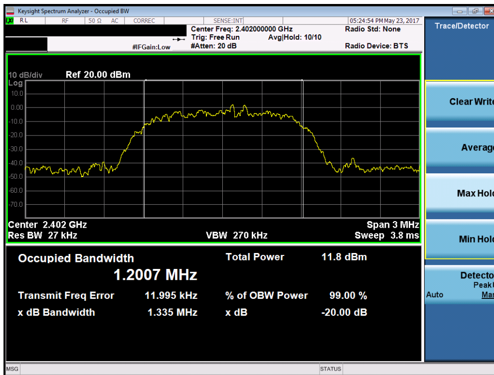
Plot 7-4. 20dB Bandwidth Plot (Bluetooth, 2Mbps – Ch. 0)
