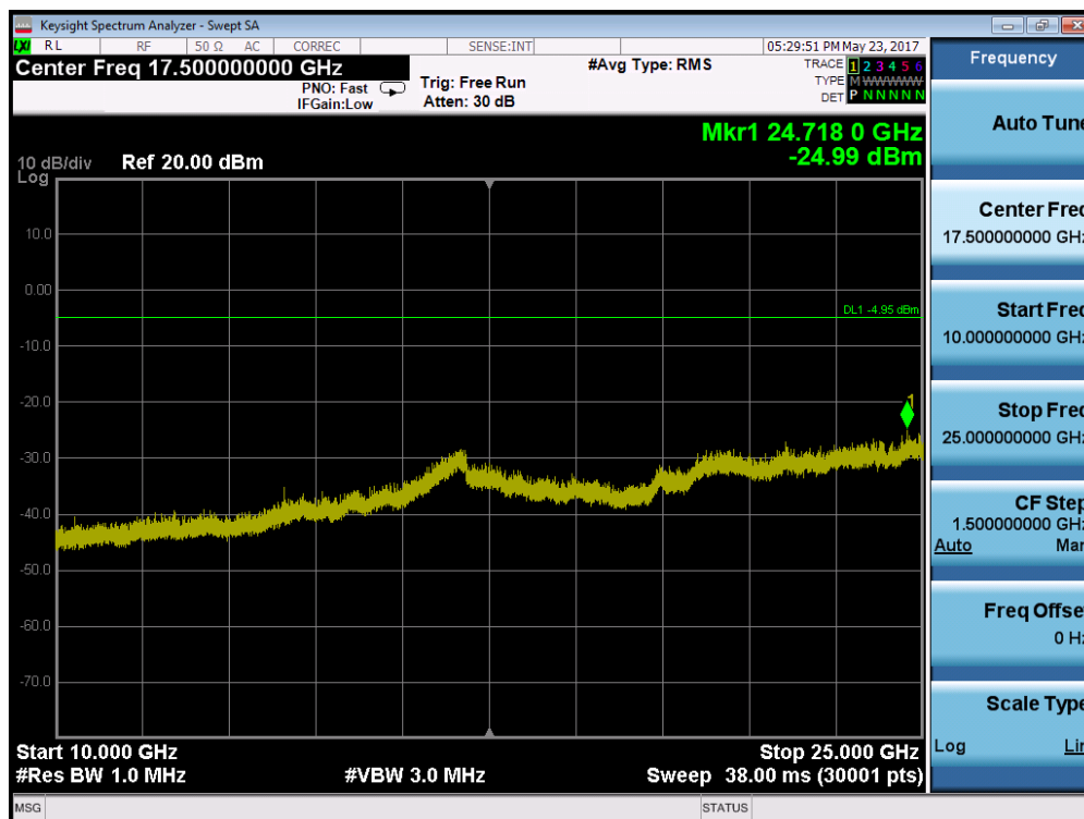
Plot 7-39. Conducted Spurious Plot (Bluetooth, 1Mbps – Ch. 39)
