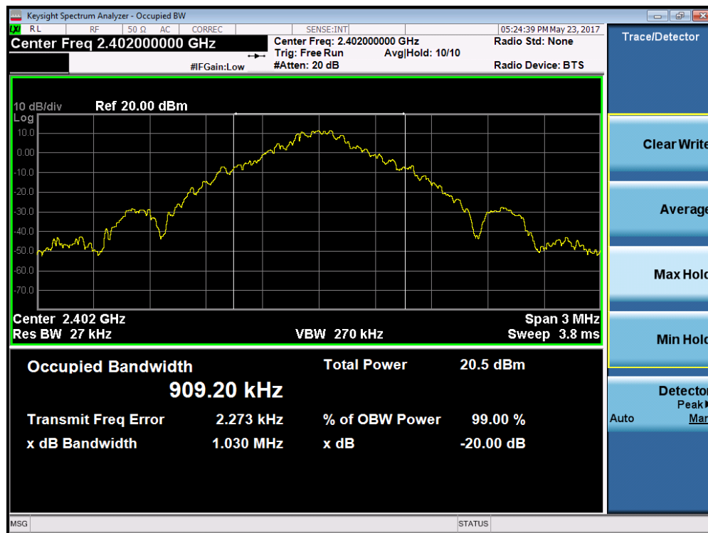
Plot 7-1. 20dB Bandwidth Plot (Bluetooth, 1Mbps – Ch. 0)
