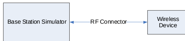
Figure 9-3 Power Measurement Setup
