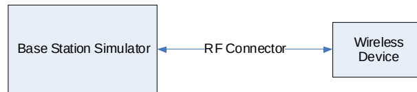
Figure 9-2 Power Measurement Setup
