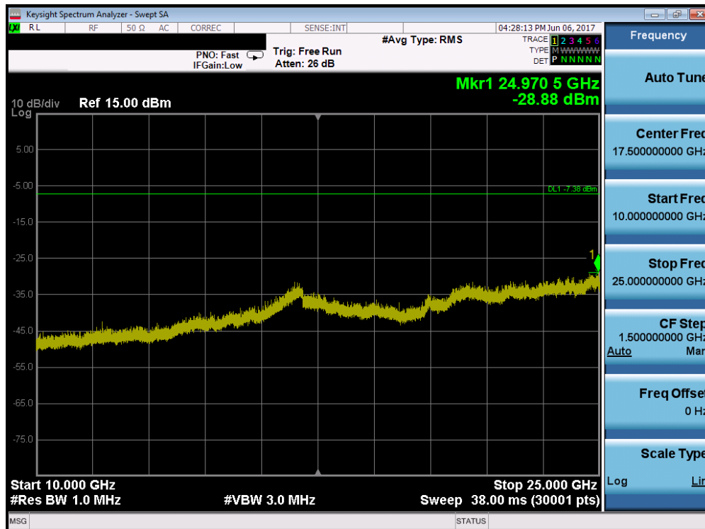
Plot 7-37. Conducted Spurious Plot (Bluetooth, 1Mbps – Ch. 0)
