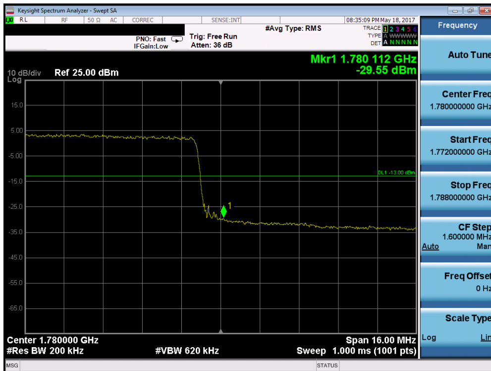
Plot 7-211. Upper Band Edge Plot (Band 66 – 20.0MHz QPSK – RB Size 100)
