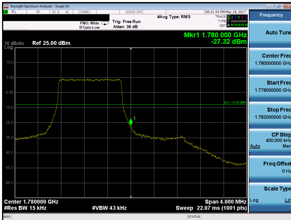
Plot 7-201. Upper Band Edge Plot (Band 66 – 1.4MHz QPSK – RB Size 6)
