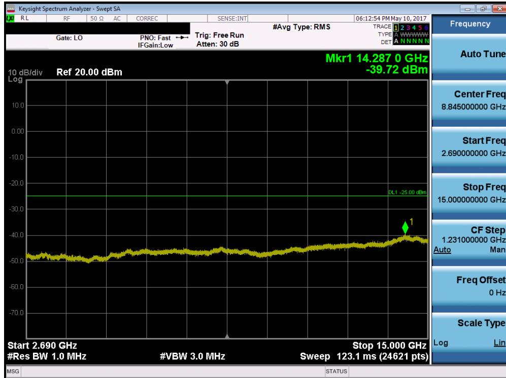
Plot 7-146. Conducted Spurious Plot (Band 41 – 20.0MHz QPSK – RB Size 1, RB Offset 0 – Mid Channel)
