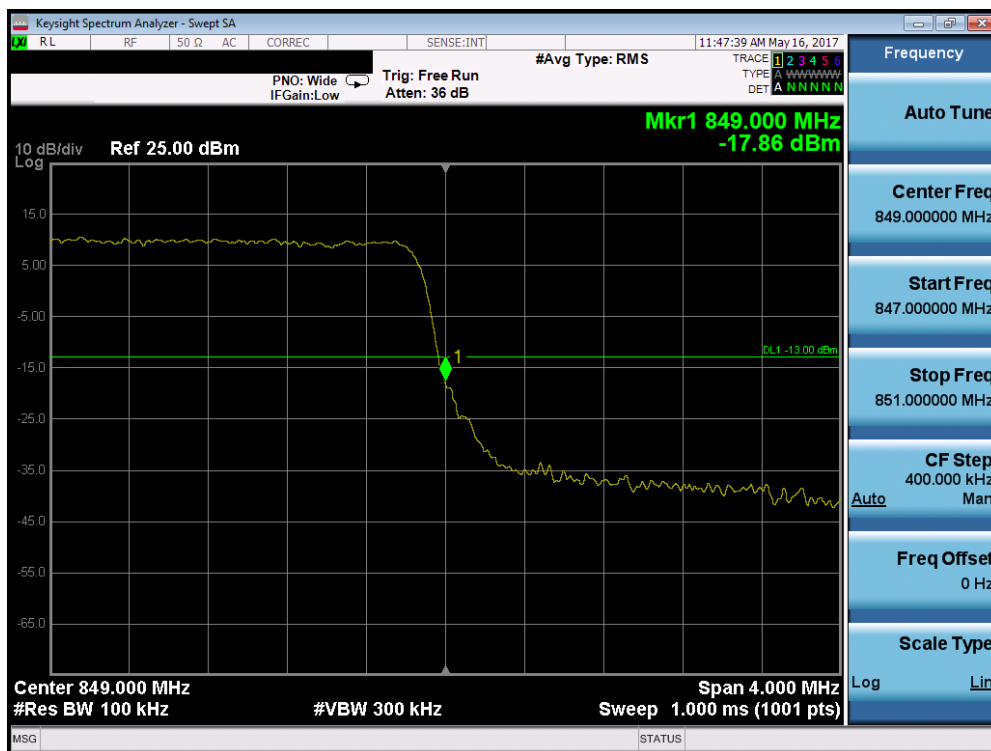
Plot 7-170. Upper Band Edge Plot (Band 5/26 - 3.0MHz QPSK - RB Size 15)
