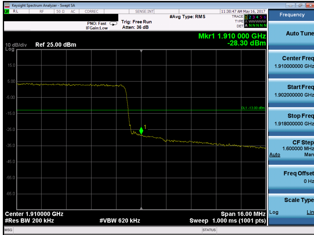
Plot 7-235. Upper Band Edge Plot (Band 2 – 20.0MHz QPSK – RB Size 100)
