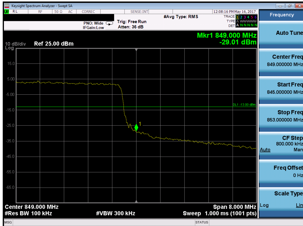
Plot 7-174. Upper Band Edge Plot (Band 5/26 – 10.0MHz QPSK – RB Size 50)
