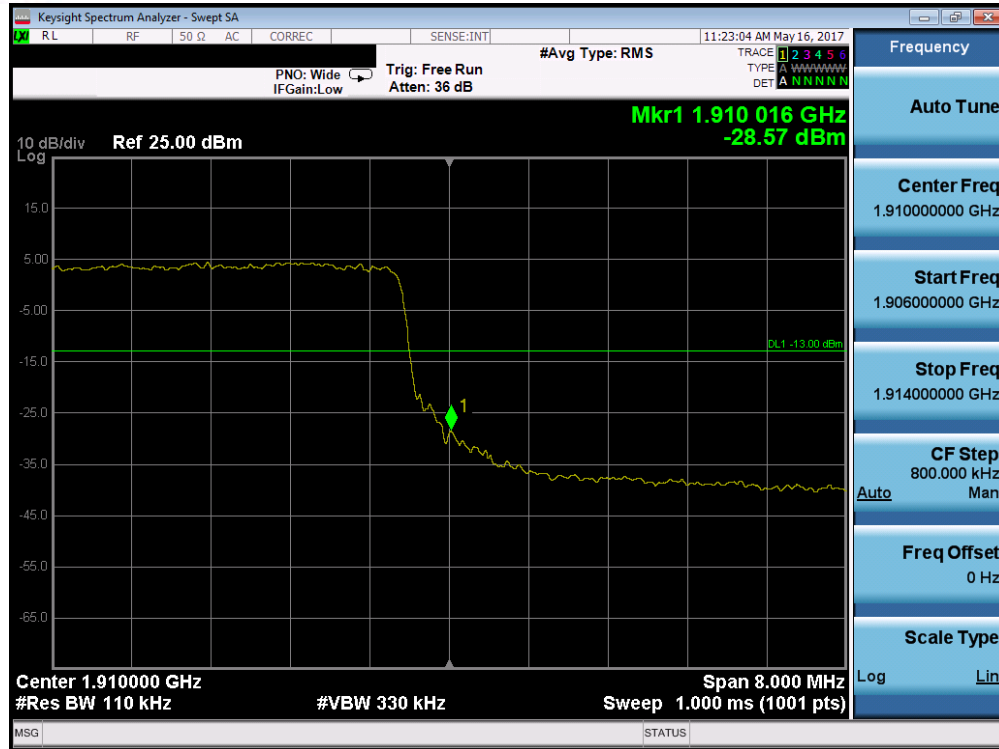
Plot 7-227. Upper Band Edge Plot (Band 2 – 10.0MHz QPSK – RB Size 50)
