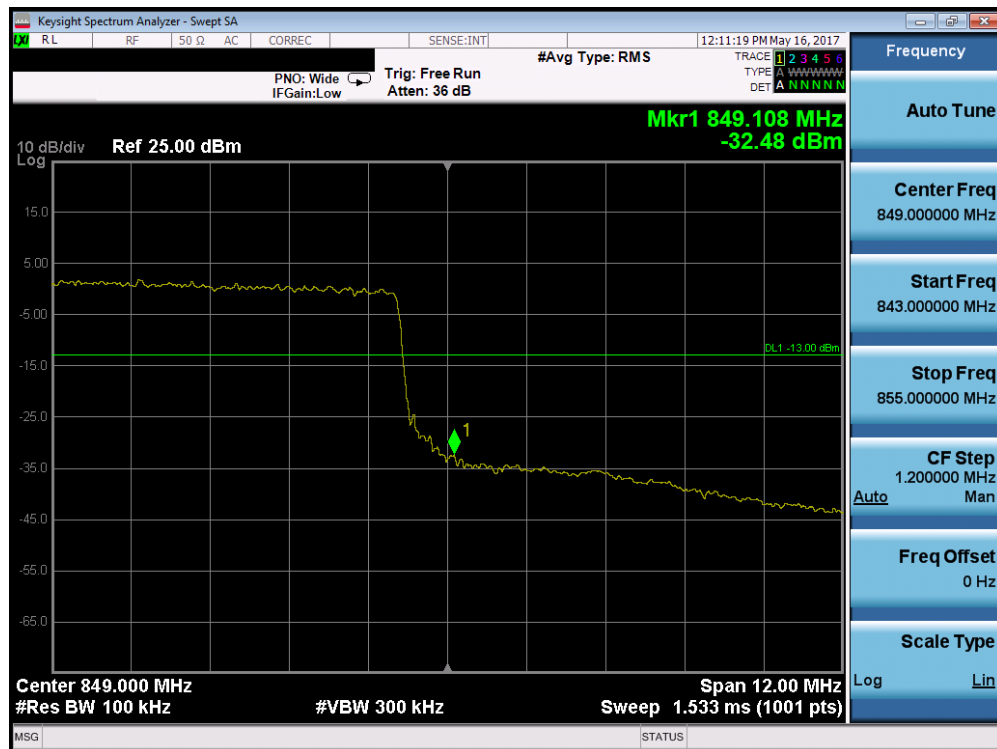
Plot 7-176. Upper Band Edge Plot (Band 26 – 15.0MHz QPSK – RB Size 75)
