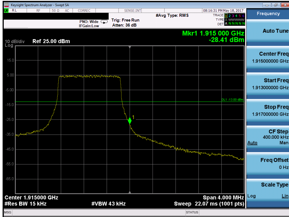
Plot 7-237. Upper Band Edge Plot (Band 25 – 1.4MHz QPSK – RB Size 6)
