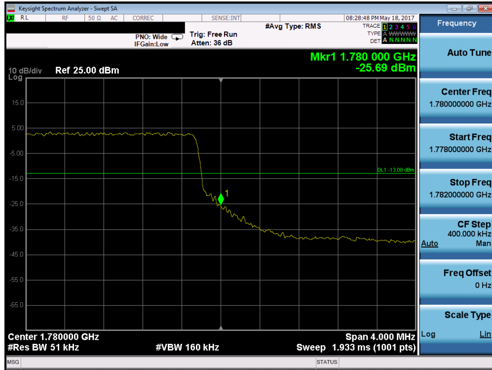
Plot 7-205. Upper Band Edge Plot (Band 66 – 5.0MHz QPSK – RB Size 25)
