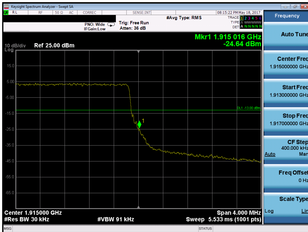
Plot 7-239. Upper Band Edge Plot (Band 25 – 3.0MHz QPSK – RB Size 15)
