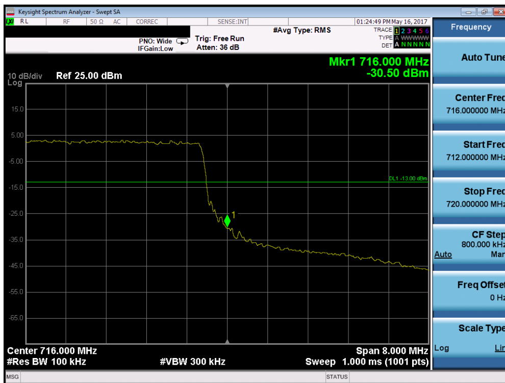
Plot 7-158. Upper Band Edge Plot (Band 12/17 - 10.0MHz QPSK - RB Size 50)
