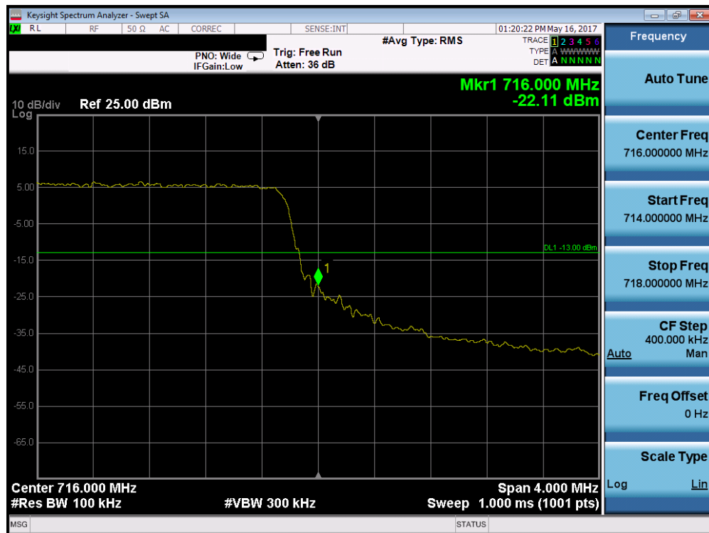
Plot 7-156. Upper Band Edge Plot (Band 12/17 – 5.0MHz QPSK – RB Size 25)
