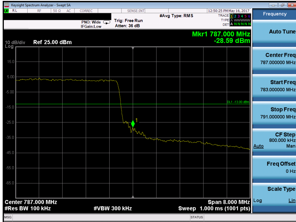
Plot 7-165. Upper Band Edge Plot (Band 13 – 10.0MHz QPSK – RB Size 50)
