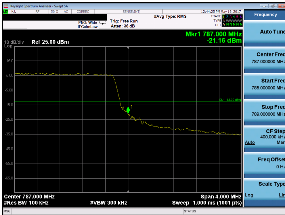
Plot 7-161. Upper Band Edge Plot (Band 13 – 5.0MHz QPSK – RB Size 25)
